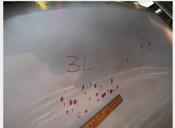
Poren in Peltonlaufrad
